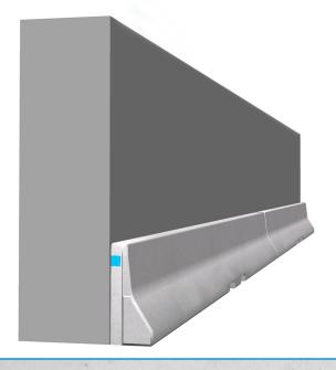
The free standing system REBLOC 80XW\_8 has been designed for the application along vertical (tunnel) walls. Thanks to its asymmetric shape, it can be positioned seamlessly along already exisiting tunnel walls. Due to the low system width valuable space keeps remaining and a sufficient width of the traffic lanes is ensured.
